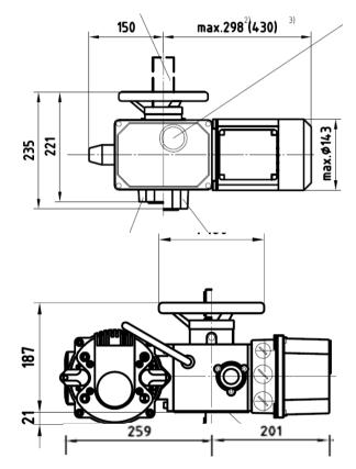
dimensions CM vs. AB3 CSC [L x B x H] [298 x 332 x 216] vs. [460 x 448 x 208]
